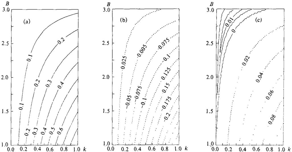
Fig. 8. The phase speed as functions of  $k$  and  $B$  for (a) modified Kelvin wave ( $K^*$ ), (b) modified Rossby wave ( $R_1^*$ ) and (c) modified Rossby wave ( $R_2^*$ ). In the computation,  $E=0.015$  and a steady boundary-layer is assumed.
