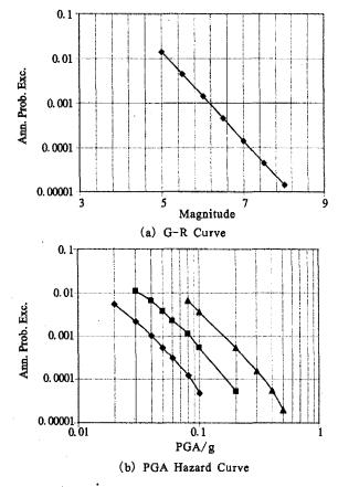
Fig. 4 Gutenburg-Ritcher (a) and PGA (b) hazard curves for a site 40 km from a line source(Square; median; diamond; median - σ<sub>ln.y</sub>; triangle; median + σ<sub>ln.y</sub>).
