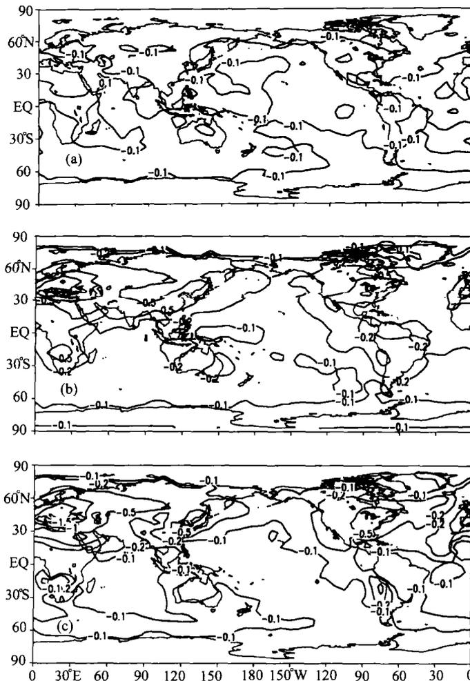
Fig. 3. C97 annual mean radiative forcing ( $\text{W/m}^2$ ) due to natural sulfate (a), total sulfate (b), and the external mixture of total sulfate and soot (c).
