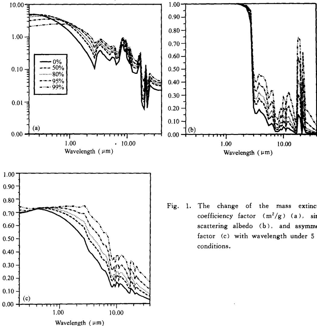
Fig. 1. The change of the mass extinction coefficient factor ( $\text{m}^2/\text{g}$ ) (a), single scattering albedo (b), and asymmetry factor (c) with wavelength under 5 RH conditions.
