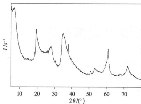
Fig.1 X-ray diffraction pattern of  $Mg_{2.7}Li_{0.3}Si_4O_{10}(OH)_2$
