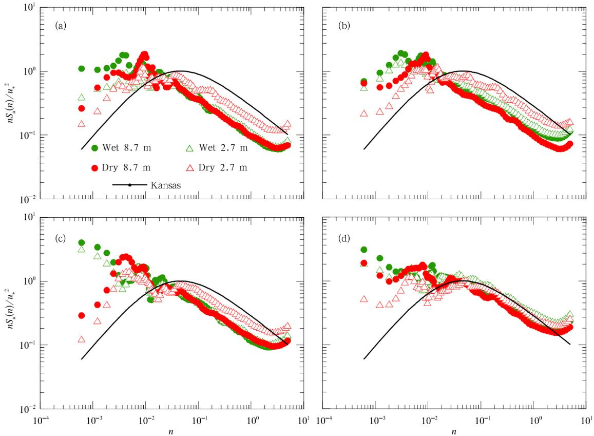
**Fig. 3.** The  $u$  spectra versus natural frequency for the irrigated case (5–7 August) and the non-irrigated case (11–13 August) on two levels (2.7 and 8.7 m) at (a) 1000, (b) 1200, (c) 1400, and (d) 1700 LT.
