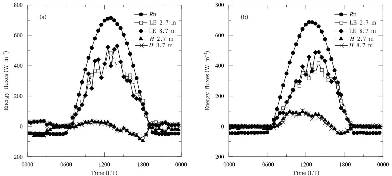
**Fig. 1.** Diurnal variations of energy fluxes ( $R_n$ : net radiative,  $H$ : sensible heat flux, and LE: latent heat flux) on (a) August 5 (an irrigated day) and (b) August 11 (a non-irrigated day).
