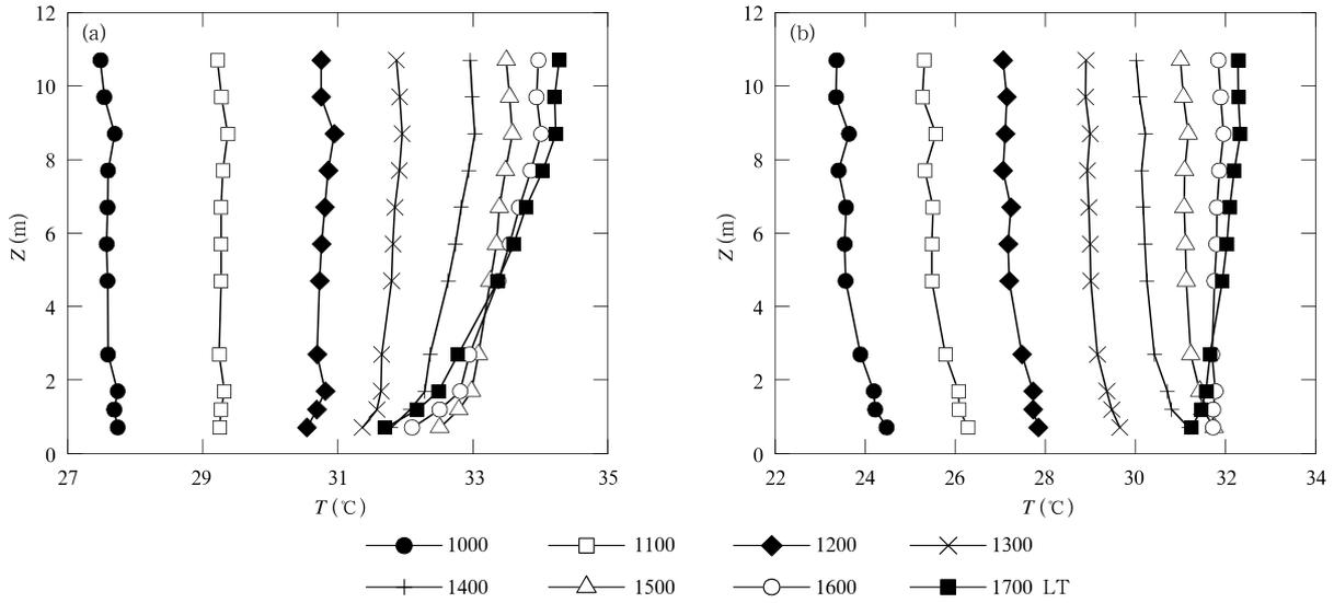
**Fig. 2.** Air temperature profiles at different times (LT) on (a) August 5 (the irrigated day) and (b) August 11 (the non-irrigated day).
