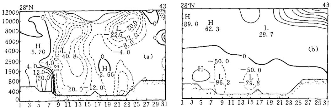
Fig. 5.  $(MPV)_y$  and  $(MPV)_z$  meridional sections along  $x = 19$  at 0000 GMT July 1, respectively in (a) and (b). Solid line:  $\geq 0$ ; dashed line:  $< 0$ ; unit:  $10^{-8} \text{ m}^2 \text{ K s}^{-1} \text{ kg}^{-1}$ .
