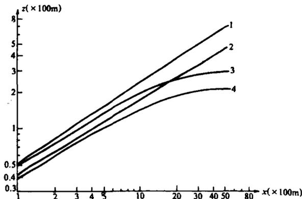
Fig. 3. Effect of ambient turbulence on plume trajectory and terminal rise height. 1:  $\delta_1 = 0$ ,  $\delta_2 = 0$ ; 2:  $\delta_1 = 1$ ,  $\delta_2 = 0$ ; 3:  $\delta_1 = 0$ ,  $\delta_2 = 1$ ; 4:  $\delta_1 = 1$ ,  $\delta_2 = 1$ .
