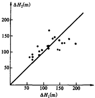
Fig. 1. Comparison between the observed values ( $\Delta H_1$ ) of plume rise tests in Xuzhou Power Plant and the calculated values ( $\Delta H_2$ ) of formula (16).
