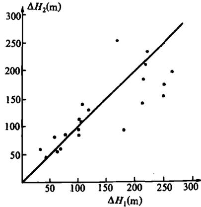
Fig. 2. Comparison of the observed values from the foreign plume rise tests with the calculated values of formula (16).
